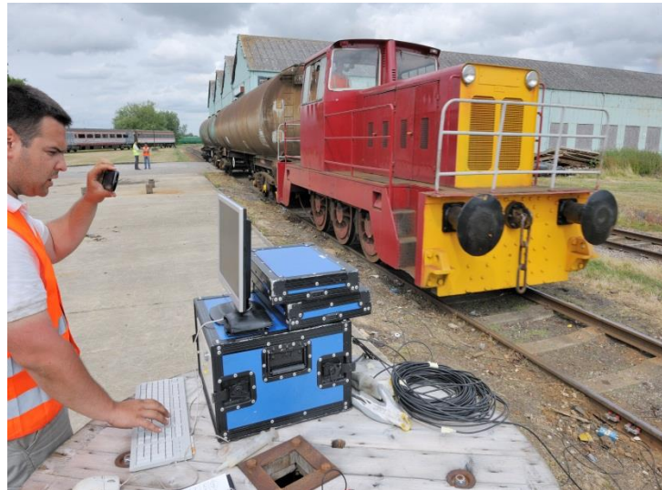
Figure 6.4. Crack growth investigation by ultrasonic (copyright TWI)
