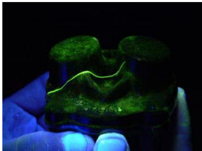
Figure 4.2. Liquid penetrant used to detect crack in parts
