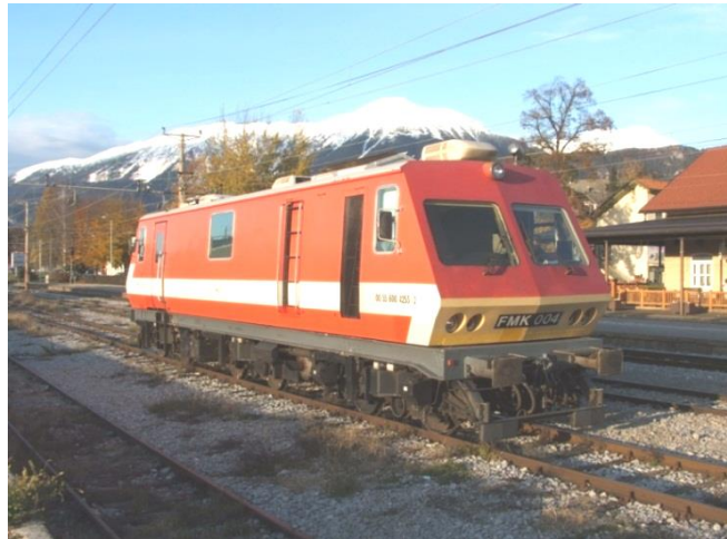
Figure 6.1. Example of track geometrical measuring car (copyright MÁV Co)
