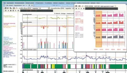
Space and time based graphical analysis of track geometry data
