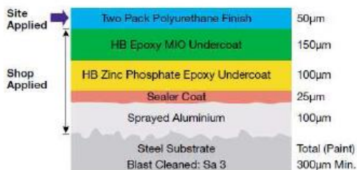
Figure 8-12 Example of high performance duplex coating system on steel substrate (CORUS 2005).
